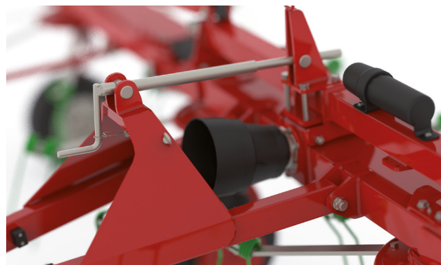
Mechanical working angle adjustment. Standard on the G4 520 PTH
